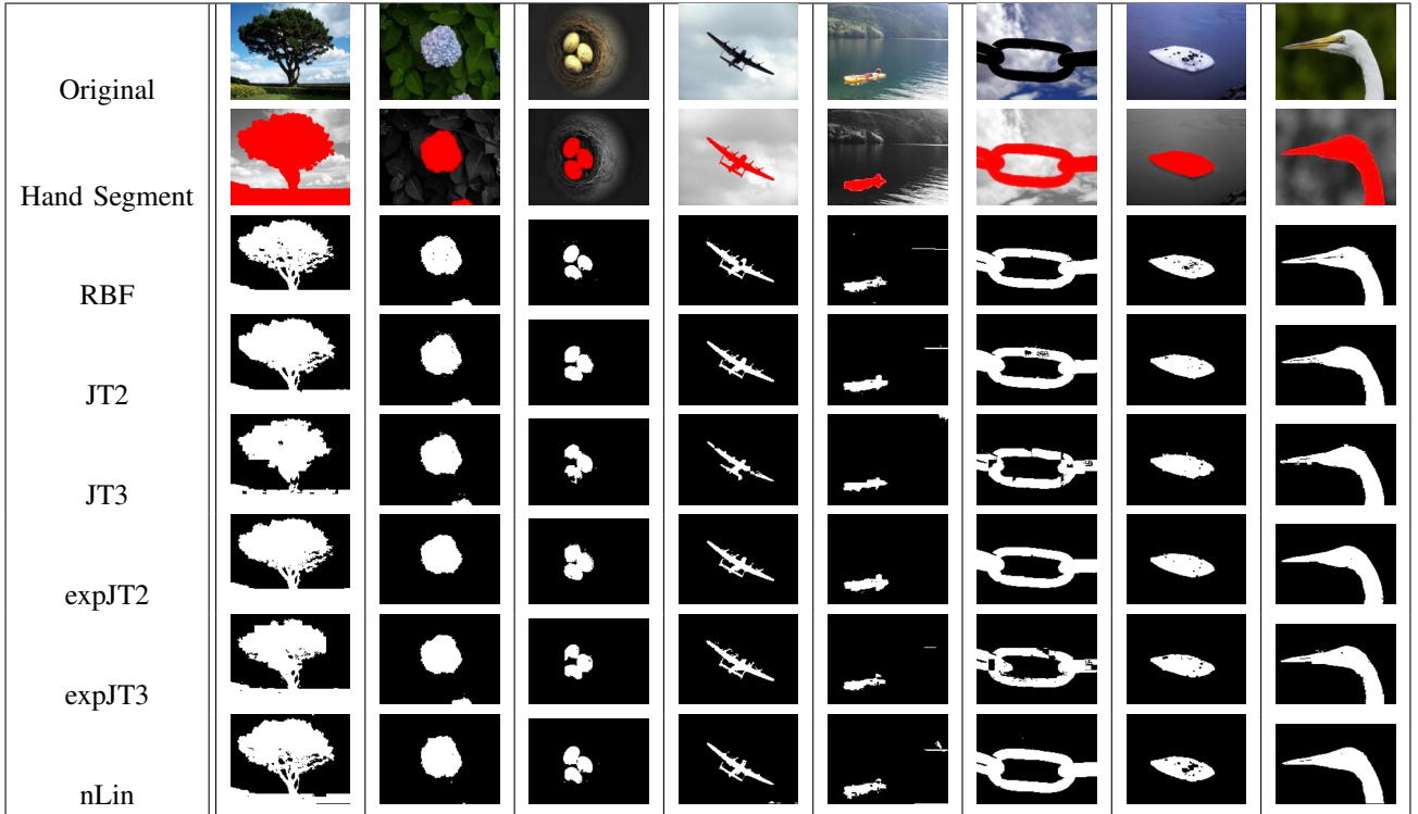
Fig. 4. Segmentation of images using spectral clustering with Gaussian and Jensen-type kernels.
