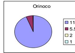
**Figure 5(b):** Lucent Orinoco Silver card - most of the packets at 11Mbps and 5.5 Mbps rates
