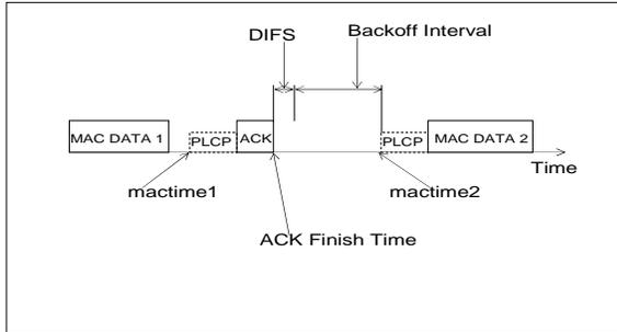
**Figure 1:** Illustration of backoff interval calculation
