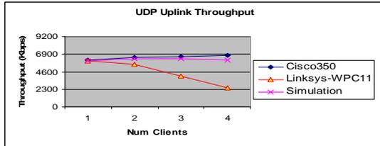
Figure 7: Inaccuracy of Throughput Prediction Tools
