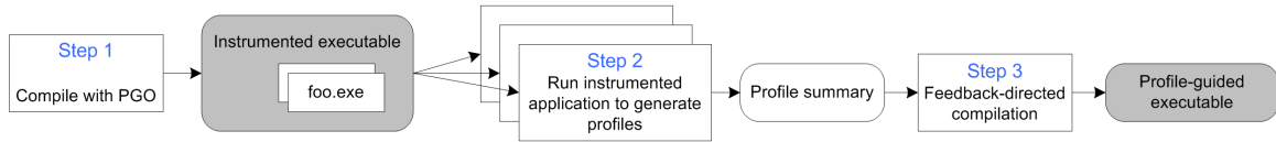
Figure 1.2: Overview of compile-profile-recompile cycle that generates binaries tuned to a specific program behavior.
