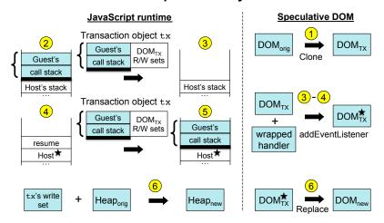
(b) Corresponding actions within the Transcript runtime system for a trap/return.
