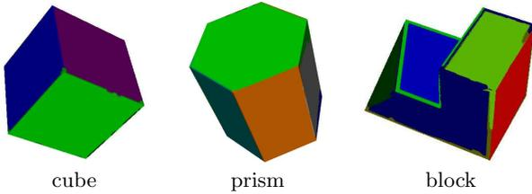
**Fig. 8** Segmentation of CAD models. Edge lengths in the  $k$ -nearest neighbor graph and in the graph of supernodes are modified before applying the multiphase segmentation process.
